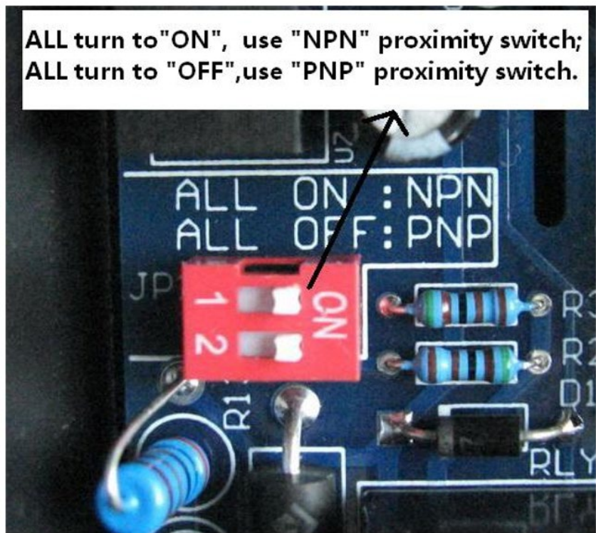
Figure 3.8 The proximity switch view upon voltage divide board
