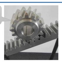
Step4: Reinstall the motor of the Y2axis; Move the motor following the direction of arrow and ensure the rack and gears are meshing.
