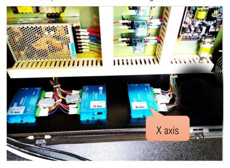
If X-axis drive damaged; Switch the alarm driver to the Y-axis driver-Beam axis; Need remove the motor for the Y1 and y2 axes; --Then test;
