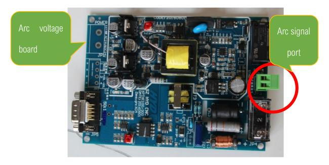
If 【arc signal port】 circuit is in open circuit, PIs check arcon signal circuit is open or not. The arcon signal circuit is marked by red line. Recover it if you confirmed it is in open circuit.
