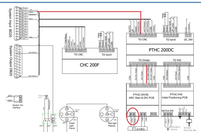
If press 【ARCON TEST】 Button, 【ARCON】 light on and arcon signal circuit works well, then check "To divider" port:
