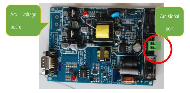
If **【**arc signal port **】** circuit is in open circuit, PIs check arcon signal circuit is open or not. The arcon signal circuit is marked by red line. Recover it if you confirmed it is in open circuit. Check the wiring with reference to the circuit diagram:
