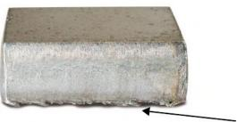
**Top spatter:** A light spatter of molten material collects on the top edges of the cut. Usually, this spatter is inconsequential and is most common with air plasma.
