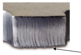
Low-speed dross: A bubbly or globular accumulation of molten material attaches and hardens along the bottom edge of the cut. In addition, vertical lag lines may be present; dross is easy to remove and flakes off in large chunks.
