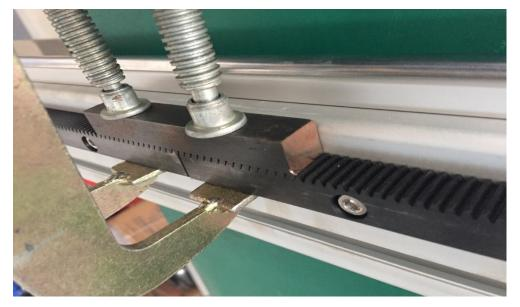
3.Screw in the bolt on B rack, which was released in step 1.
