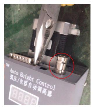
Step 4: Take off the shell screws of THC as pic ;
