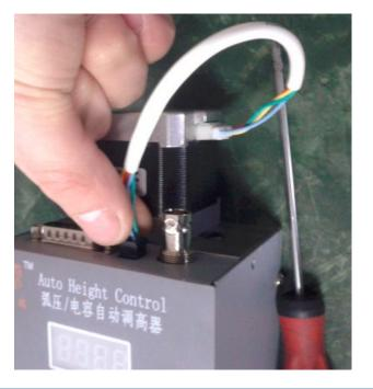
Step 3: Take off the two nuts of 15-pin plug and Capacitor connector as pic;
