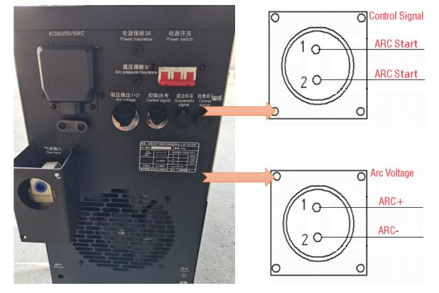
ℜ Refer to the following table when connecting the Aricut60/105/120 to CNC controller with cable.
