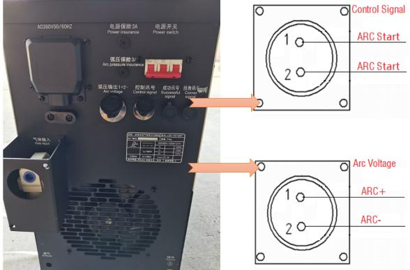
畿 Refer to the following table when connecting the Aricut60/105/120 to CNC controller with cable.
