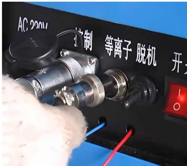
➔ Signal connection of ARC+/ARC-
