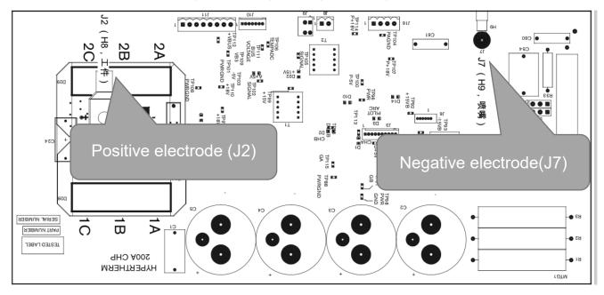
NOTES 1: Positive electrode (work--J2) of Plasma power is connected the ground wire. and check it by multimeter. If \[ \text{work} \text{-J2} \] is not connected the ground wire, please find the other port.
