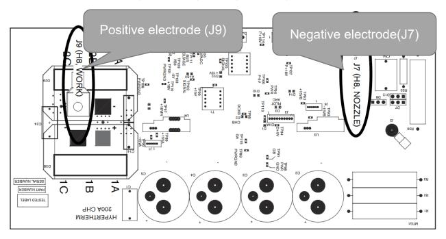
NOTES 1: Positive electrode (work—J9) of Plasma power is connected the ground wire. and check it by multimeter. If **\( \)** work-J9 **\)** is not connected the ground wire, please find the other port.
