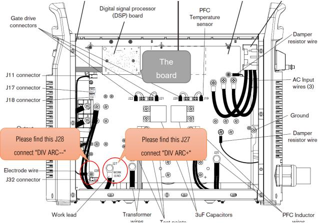
NOTES 1: Positive electrode (J27) of Plasma power is connected the ground wire. and check it
