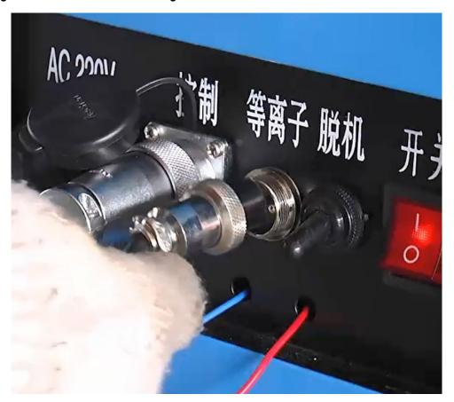
→ Signal connection of ARC+/ARC-
