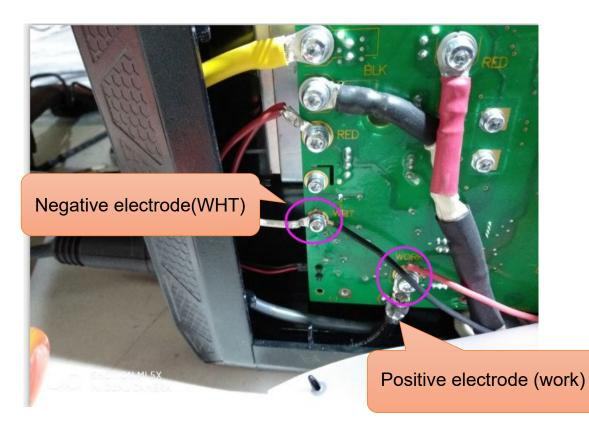
NOTES 1: Positive electrode (work) of Plasma power is connected the ground wire. and check
