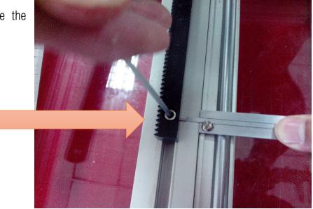
Step 2: Fixed the second rack, at the same time use the third rack mesh ensure two rack of meshing
