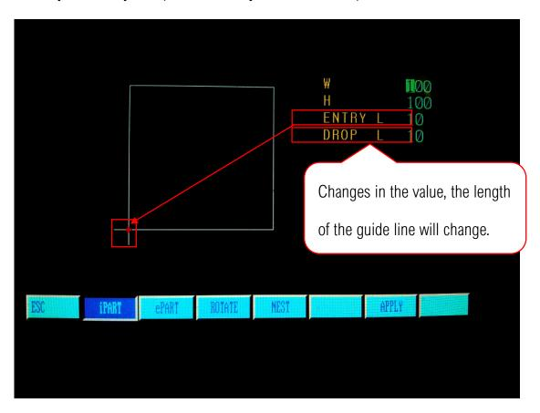
**TENTRY L** : means guide length, in order to avoid the work piece been damaged at the begin of cutting, it need some distance to start cutting the work piece.
