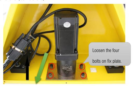
Ensure the rack and gears are separated. Then tighten the one bolts on fix plate
