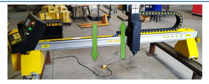
Step3: Reinstall the motor of the Y1 axis; Move the motor following the direction of arrow and ensure the rack and gears are meshing. Then tighten the bolts on fix plate.
