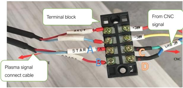
Check CNC of ARCON light is on or no and Check C and D from CNC side, if connected at the same time, the ARCON indicator light, means that the CNC can send signal of arc start. Otherwise, please contact us for further investigation of the program;
