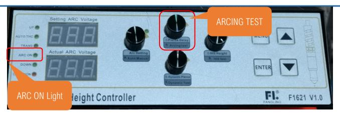
Solution: Keep pressing 【ARCING TEST】 Button on the THC panel, If 【ARCON】 light is on, At the same time, there is has an output arcing signal on the THC board.
