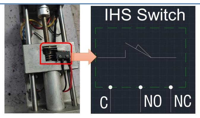
NOTE: Open the lifting cover; The iron sheet on the IHS switch is deformed, which can also cause problems.
