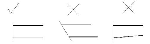
When doing the rack joint, take another rack to make the corresponding, then it can make sure the clearance, at last fixed the rack.
