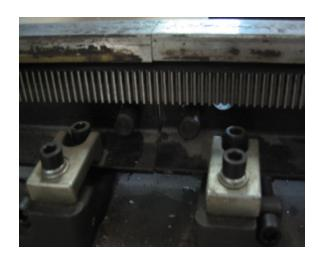
2: Fixed the Rack to the 24KGS Steel track, and install the Track Adjustment.
