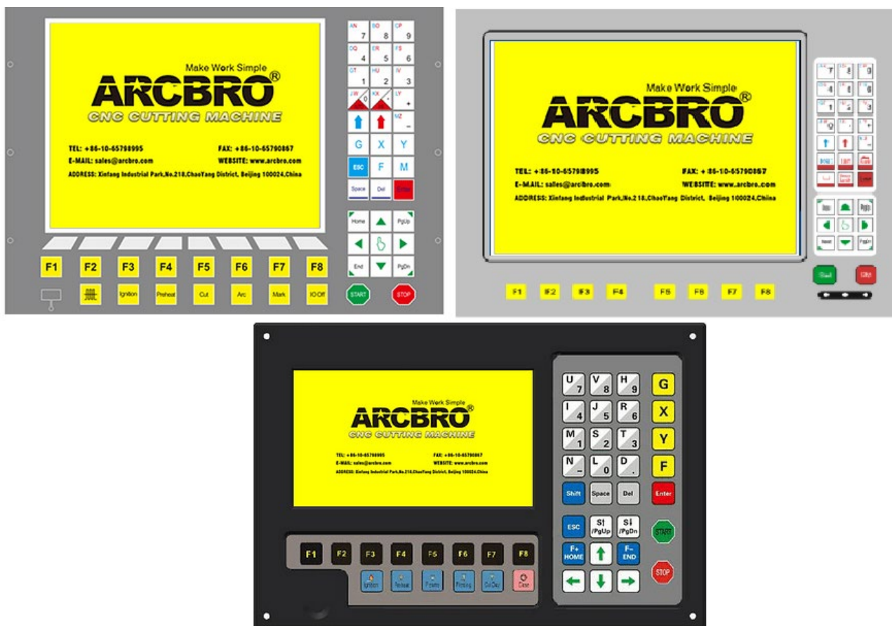
Fig 2.1 F2000 Series System Board
