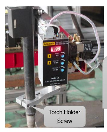
Usually: The distance between the torch nozzle of and the holder is about 150mm.
