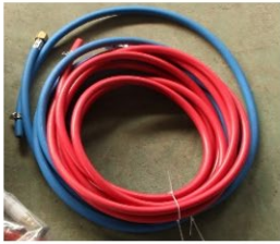
8. Oxygen and gas pipe-1Set
