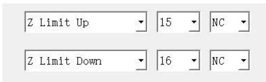
Figure 14.1 Motor Control Input Configuration
