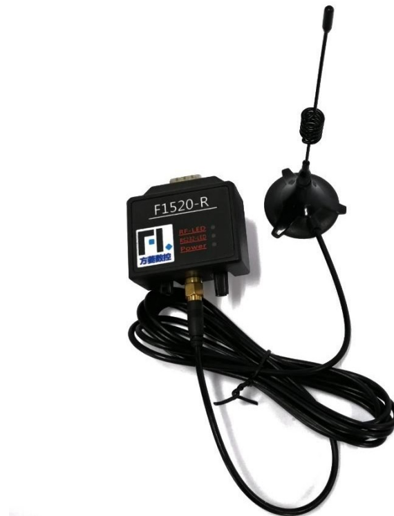
Figure 10.17 Serial Telecontroller Receiver
