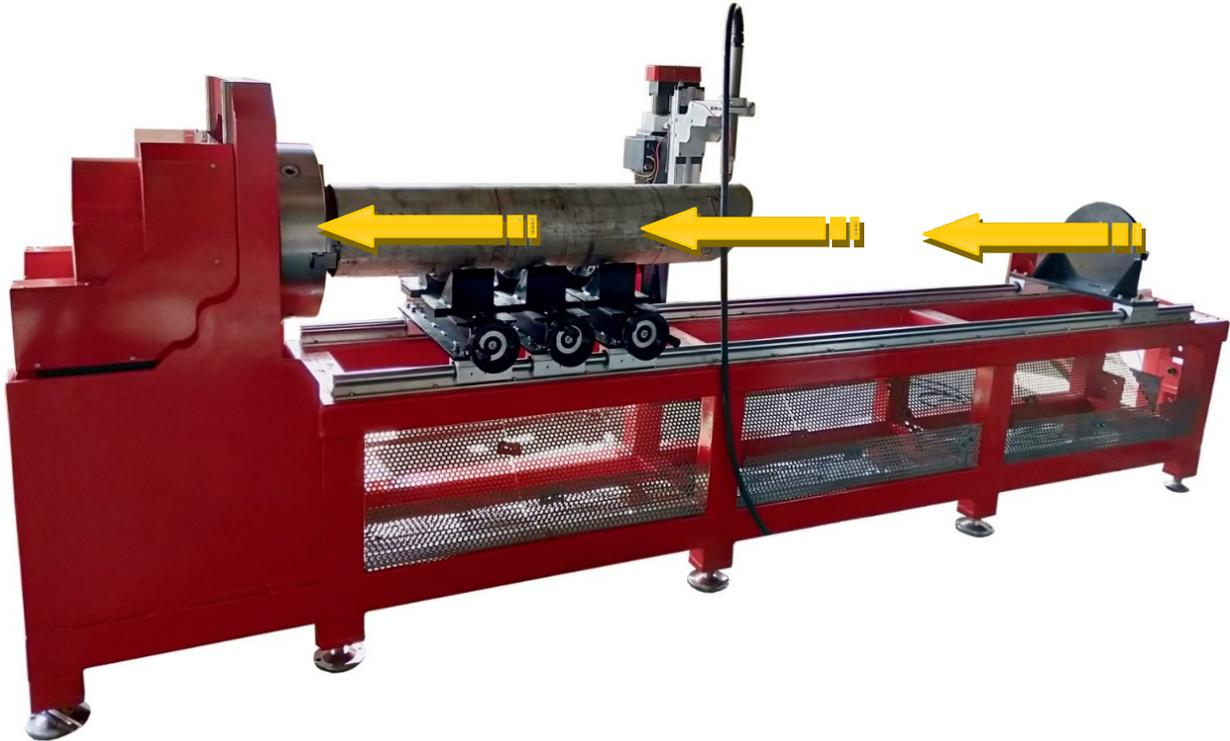
Note: The centrelines of the pipe and the centrelines of the chuck remain coincident;
