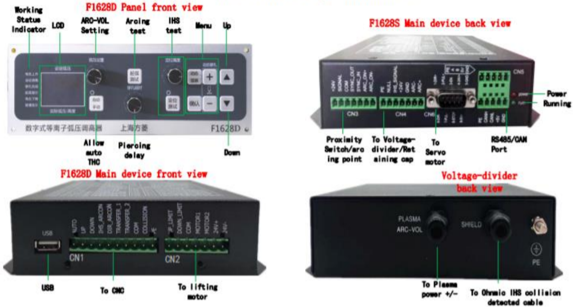
Figure 3. 12 F1628D chassis and voltage divider view
